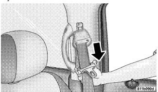
2. The seat belt latch plate is above the back of the front seat, next to your arm in the rear seat. Grasp the latch
